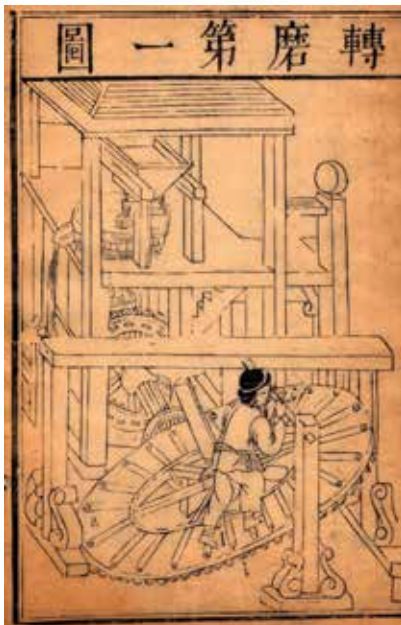
Transmission of engineering knowledge: a treadmill in the Qiqi tushuo from 1627 (left) and in Agostino Ramelli's Le Diverse et artificiose machine , 1588 (right).
