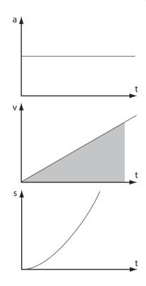
Figure 1: Derivation of the law of fall from the assumption of a constant force of gravity in classical mechanics
